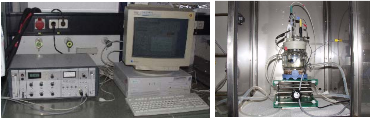
Fig. 1: potentiostat and electrochemical test cell
