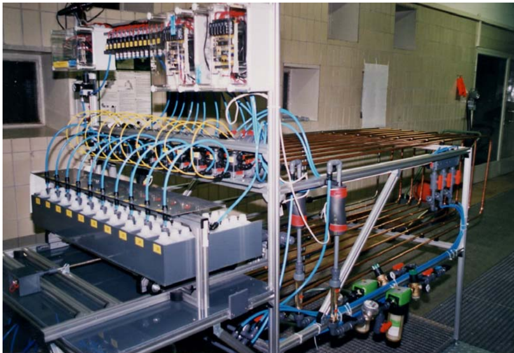
Fig. 2: Picture of a corrosion test plant according to DIN 50931-1
